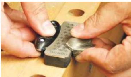
▲ The blocks allow the hones to sit flat while still allowing you to hold them firmly
